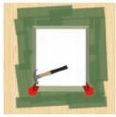
• Mechanically fasten the RED ZONE CORNER GUARDS in place.
