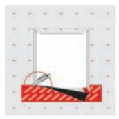
• Install bands of RED ZONE membrane, starting with the sill. Cut on both sides of the opening.
