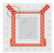
$\bullet$  Cover the  $45^\circ$  cuts in the header WRB with bands of RED ZONE membrane.
