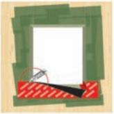
• Cut the membrane on both sides of the opening.
