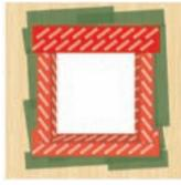
Cover the inside of the header with a band of RED ZONE membrane.
