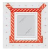
• Seal the header with a band of RED ZONE membrane to ensure the continuity of the air barrier.
