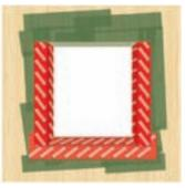
• Install a band of RED ZONE membrane inside each jamb.
