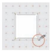
• Cut strips of WRB to cover the sill, jambs, and header of the window. Fix in place, leaving the header piece
