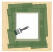
Prime plywood, OSB, and fibreglass panels with RESISTO EXTERIOR PRIMER or RESISTO H<sub>2</sub>O PRIMER to ensure proper adhesion.
